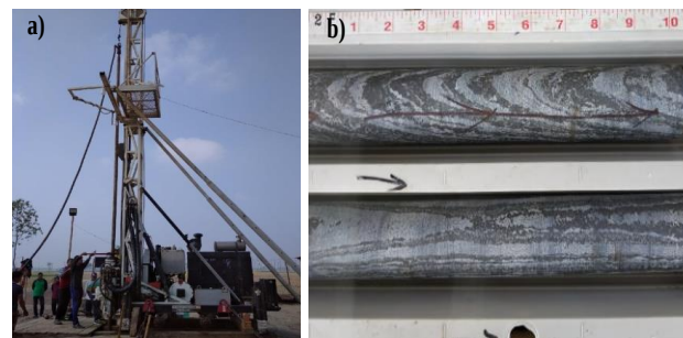
Fig. 4 Photographs showing (a) the LF Core Drill–90 drilling rig and (b) representative basement rock core samples.
