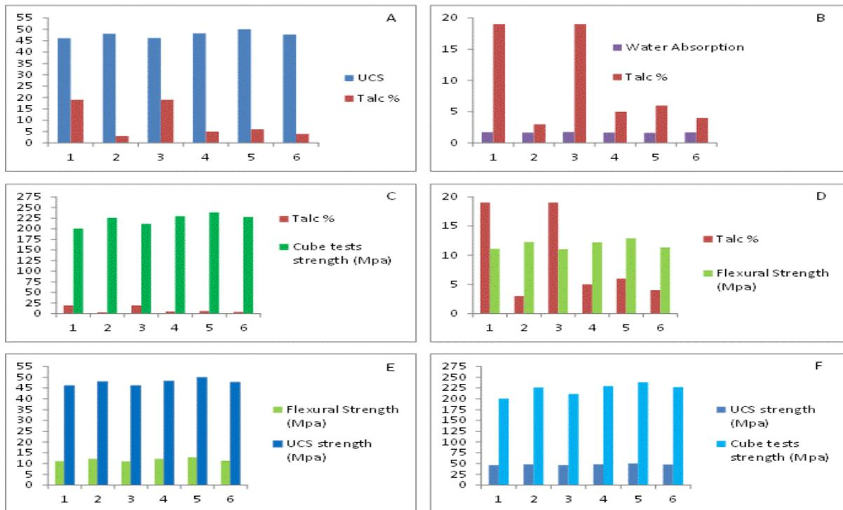
**Fig. 4** Showing the mutual relationship of mineralogy and physico-mechanical properties; Talc and UCS (A), Talc with Cube test strength and Flexure strength (B, C respectively), Talc and water absorption (D), UCS with flexure strength and Cube test strength and (E, F respectively).
