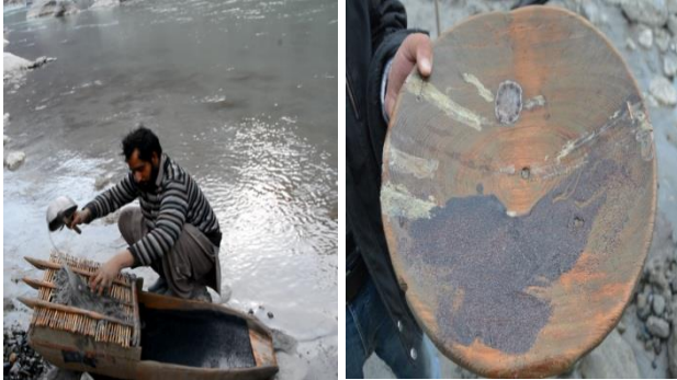
Fig. 2 Field picture showing process of placer gold extraction with shaking table and pan.
