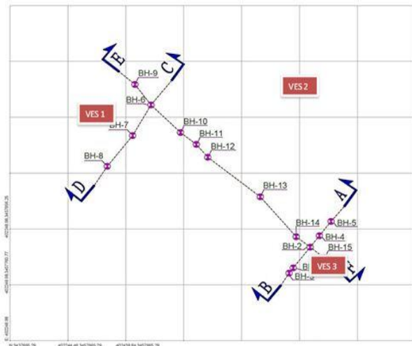
Fig. 1 Study site boreholes and VES points marked on base map.
