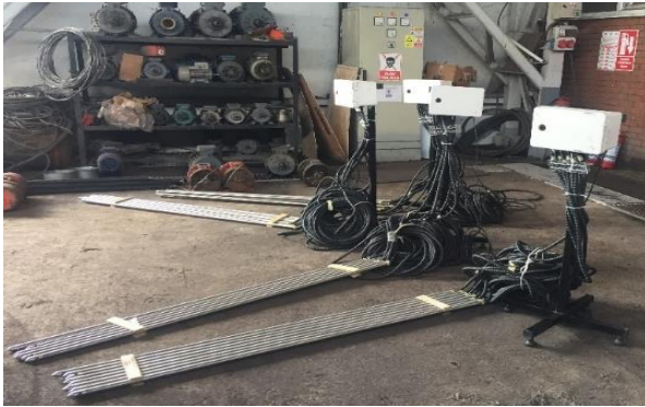
Fig. 3 Temperature measurement probes and data logger
